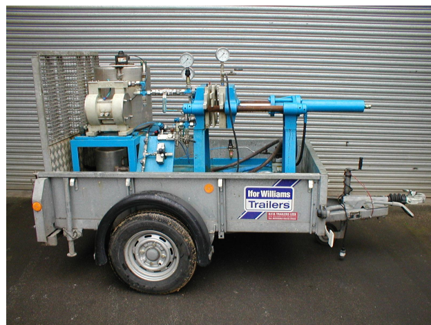
Trailer mounted self contained test rig
