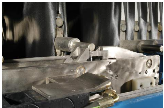
Plate Moving Mechanism with Shaker device for assisting cake discharge
